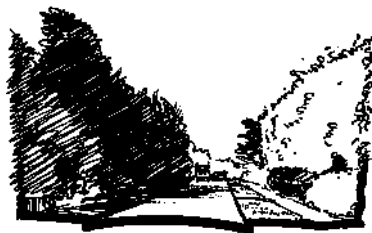
High Street, Welford-on-Avon, Avon Valley area, a primary route with (left to right) verge, carriageway, verge and footway
